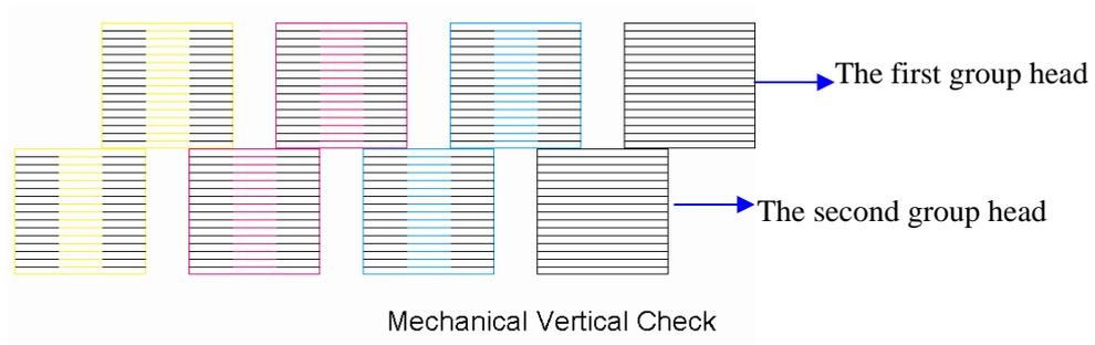
NG: If the pattern is not vertical, the operator need to do the physical position adjustment:
