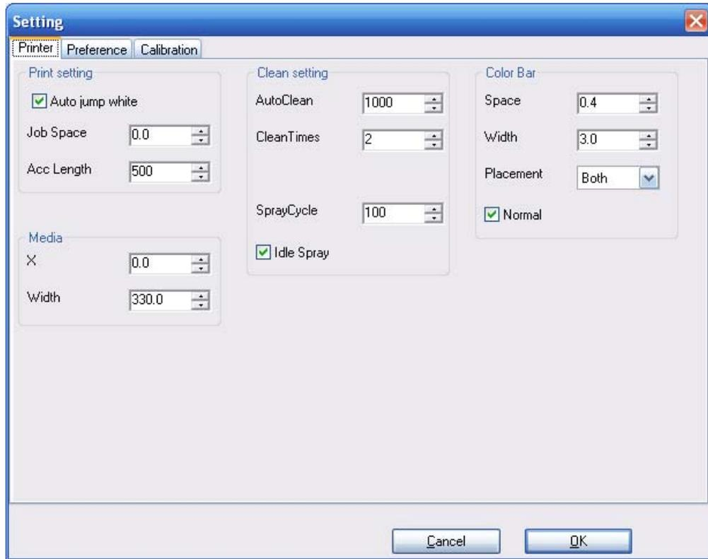
The higher the number in “clean times”, the longer the cleaning time last. Setting clean times according to the nozzle broken status, Then perform
